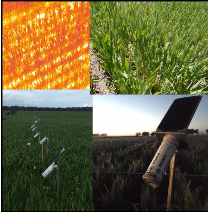
Figure 1. Left top: Thermal Imagery of wheat captured from a RPAS (FLIR TAU2 640 25mm). Right top: An example of the field of view of Arducrop V1 sensors. Left bottom: Network of Arducrop sensors deployed at the field site. Right bottom: Arducrop V1 thermal sensor.
