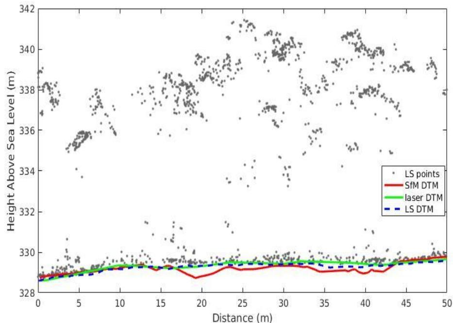
Figure 1. North South transect through the plot area showing the DTM levels extracted by the SfM (red), laser rangefinder (green) and UAV-laser scanner (LS) (blue) approaches. The image based (SfM) DTM exhibits interpolation artefacts between 20 m and 40 m which result in an under estimation of terrain height and an over estimation of tree height.
