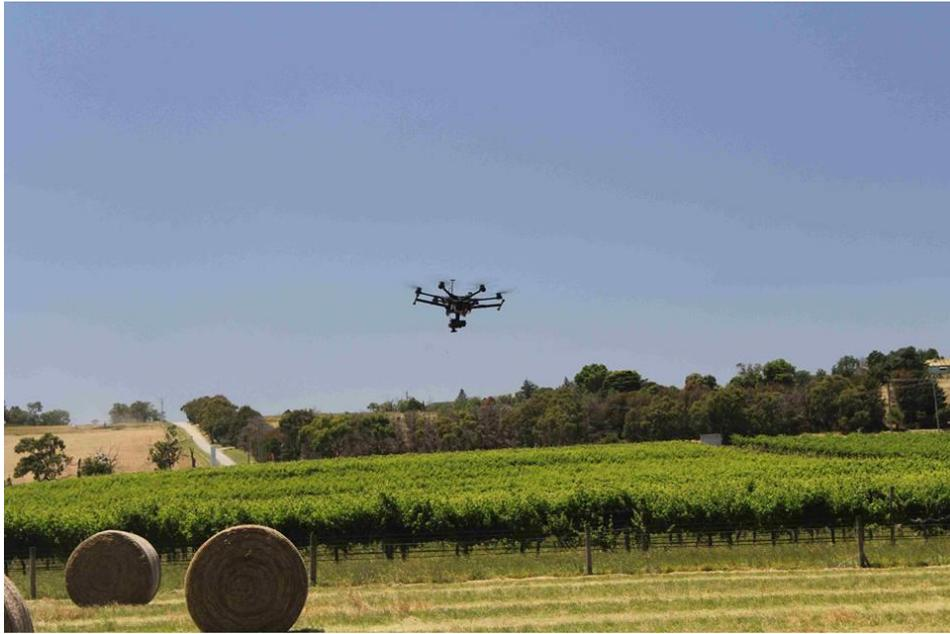
Figure 1. Multi-rotor UAV with hyperspectral camera over infested vineyard.
